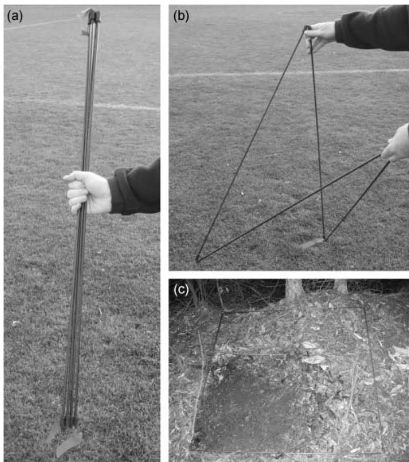
Figure 2. (a) Folded (carrying) position; (b) unfolding; (c) in use surveying leaf litter for invertebrates (note the colour flagging tape).
