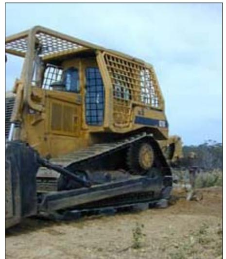
Three steps in limiting the spread of *Phytophthora cinnamomi* on tracked vehicles: first chipping off compacted soil from tracks with a crowbar, then a high pressure water spray removes general accumulation of soil (note how tracks have been lifted off the ground) and finally, at the completion of washing the dozer is lowered onto rubber tyres in preparation for loading onto a float. (Photographs by Forestry Tasmania)
