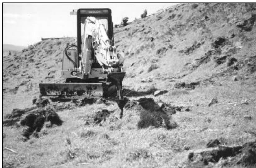
Figure 1. Ripper type and boot at end of tyne. The big clods in this photo are due to trying cultivation on an area not spot sprayed previously – the ground was considerably less lumpy on spot sprayed areas with finer tilth and better planting bed).
