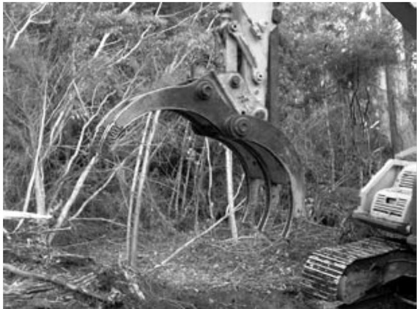
A good purpose built grab for excavator heaping designed for scooping outwards.
