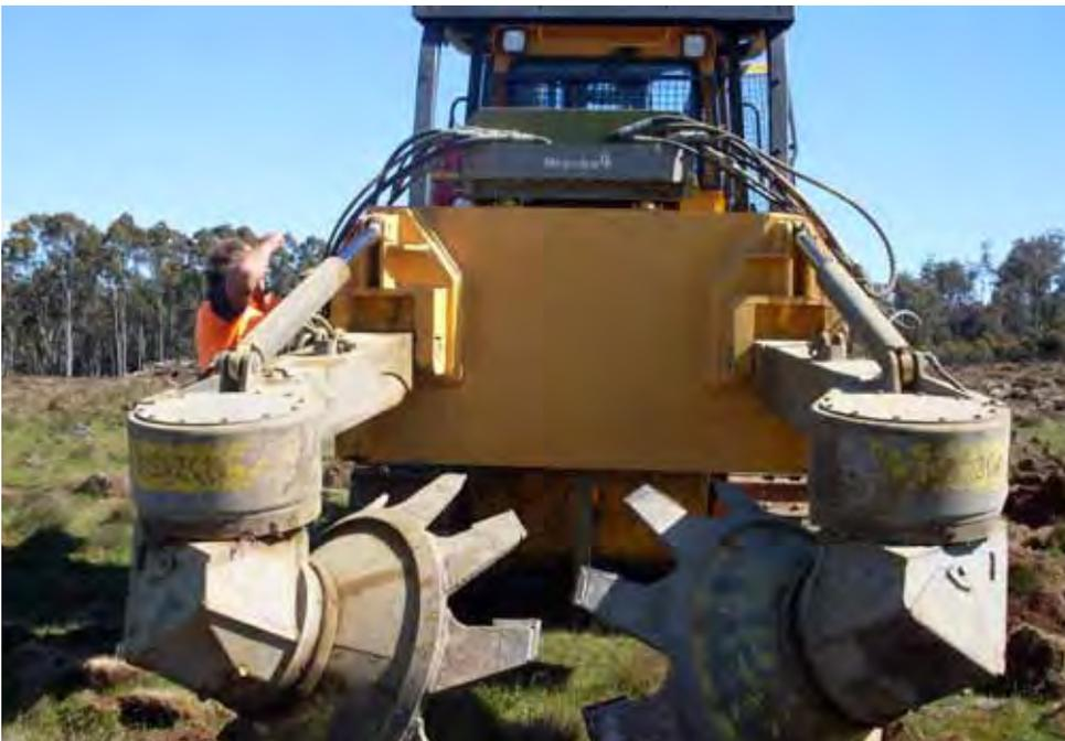
The Bracke mound plough. As all our work is in second rotation sites, this machine has the ability to straddle the stump line and place a mounded line over the existing stumps; as pine stumps break down very quickly they'll contribute of nutrients. The plough turns hydraulically, which produces a better till than the savannah plough. (photograph by Richard Shoobridge)
