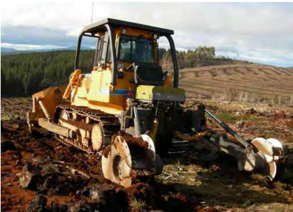
The Bracke twin spot moulder has the ability to do two mounds at a time. The on-board computer can be set to dig the spot mounds at the required spacing. Effectiveness can vary due to the presence of rocks, and sometimes the machine misses spots.
